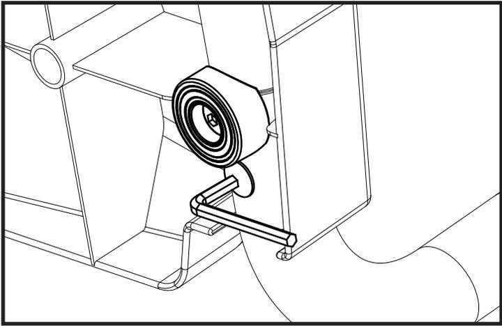
**Figure 3:** Fully tighten all Boarding Platform Bolts using the 5mm Allen Wrench.
