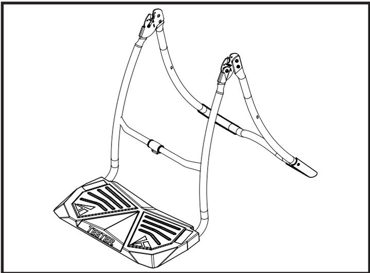
**Figure 4:** Position the assembled A-frame upright and open it on a level surface, ensuring the Boarding Platform and Rubber Feet are secure and rest evenly on the ground.
