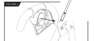
ign the black plastic part of the corresponding handle (left / right) rer the outside edge of the Hinge Plate on the A-Frame (Figure 2).
