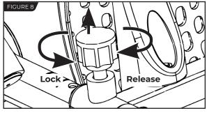
Pinlock Function - Pull out, turn counterclockwise to lock, clockwise to release
