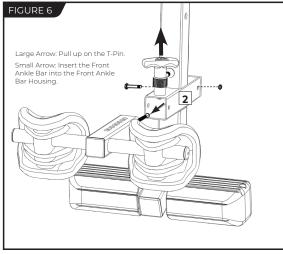
• Remove the Nut and Bolt located near the back of the Front Ankle Bar housing (Figure 6) using the wrenches provided. This will disengage the spring and cable inside the housing. **KEEP** the Nut and Bolt for use in Step 3.
